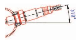
Recommended design of the mating thread in the exhaust pipe \*: THexagon > 600°C or TGas > 930°C
