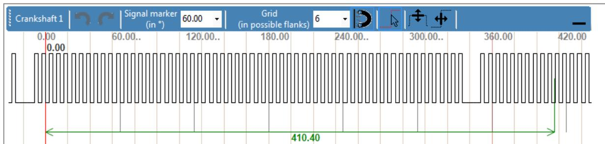
Figure 4: MicroLC Software - Illustration of crankshaft signal and editing possibilities
