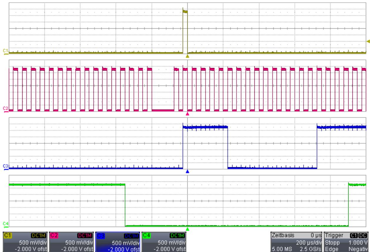
Figure 2: Illustration of the simulated crankshaft and camshaft signals shown on the oscilloscope
